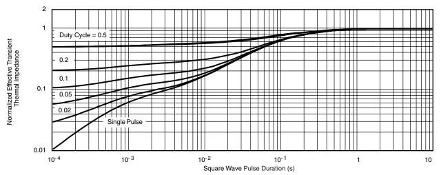
Normalized Thermal Transient Impedance, Junction-to-Foot
