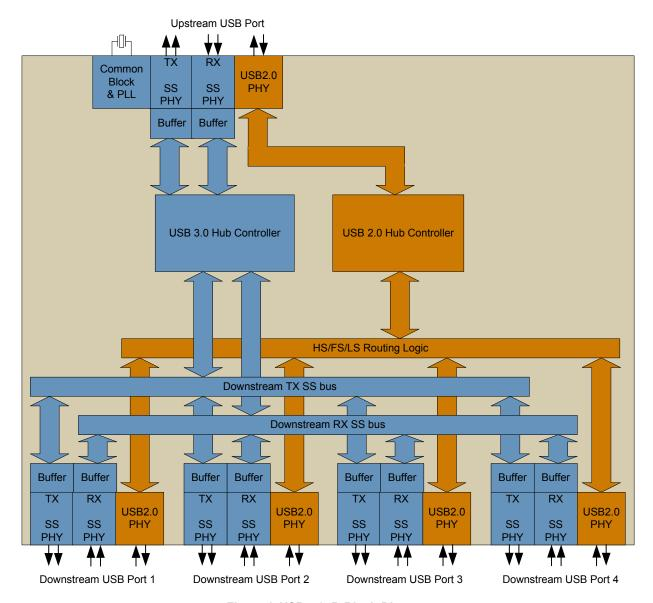
Figure 1 USB5434B Block Diagram
