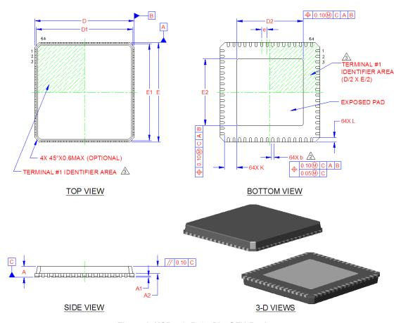
Figure 2 USB5434B 64 Pin QFN Package
