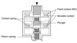
Conforms to EN60947-5-1 Direct Opening (Both NC Contacts have a direct opening mechanism.)
