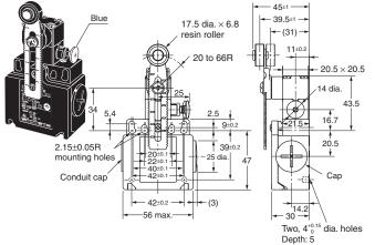
Adjustable Roller Lever, Form Lock (with Metal Lever, Rubber Roller) D4N-6□2HR
