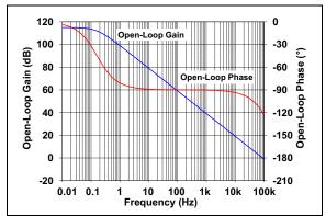
**FIGURE 2-17:** Open-Loop Gain, Phase vs. Frequency.
