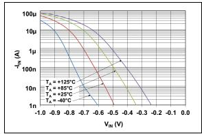
**FIGURE 2-35:** Measured Input Current vs. Input Voltage (below V<sub>SS</sub>).
