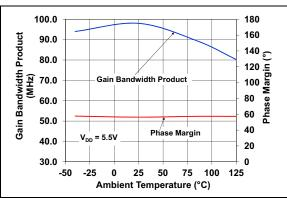
**FIGURE 2-20:** Gain Bandwidth Product, Phase Margin vs. Ambient Temperature.
