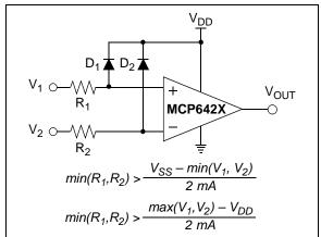
FIGURE 4-3: Protecting the Analog Inputs.
