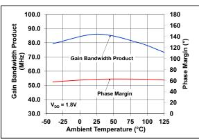
**FIGURE 2-21:** Gain Bandwidth Product, Phase Margin vs. Ambient Temperature.
