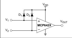
FIGURE 4-2: Protecting the Analog Inputs.
