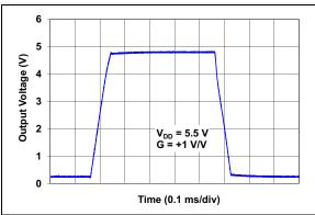
FIGURE 2-31: Large Signal Non-Inverting Pulse Response.
