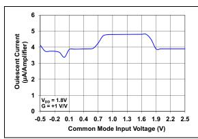
FIGURE 2-15: Quiescent Current vs. Common Mode Input Voltage.
