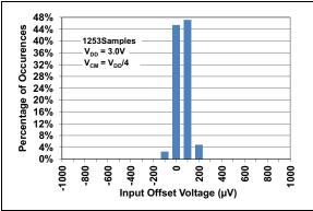
FIGURE 2-1: Input Offset Voltage.
