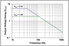
FIGURE 2-23: Output Voltage Swing vs. Frequency.
