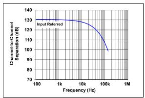
FIGURE 2-38: Channel-to-Channel Separation vs. Frequency.
