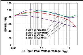
FIGURE 2-37: EMIRR vs. RF Input Peak-to-Peak Voltage.
