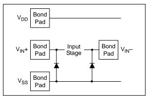
FIGURE 4-1: Simplified Analog Input ESD Structures.
