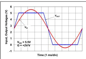
FIGURE 2-33: The MCP6421/2/4 Device Shows No Phase Reversal.
