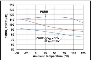
FIGURE 2-10: CMRR, PSRR vs. Ambient Temperature.
