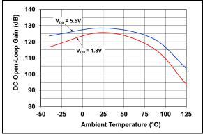
FIGURE 2-18: DC Open-Loop Gain vs. Ambient Temperature.
