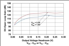
FIGURE 2-19: DC Open-Loop Gain vs. Output Voltage Headroom.
