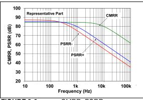
FIGURE 2-9: CMRR, PSRR vs. Frequency.
