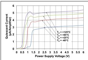
**FIGURE 2-14:** Quiescent Current vs. Power Supply Voltage.
