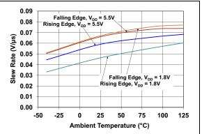
FIGURE 2-28: Slew Rate vs. Ambient Temperature.
