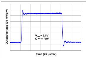
FIGURE 2-29: Small Signal Non-Inverting Pulse Response.
