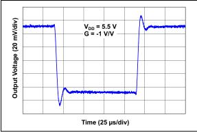
FIGURE 2-30: Small Signal Inverting Pulse Response.
