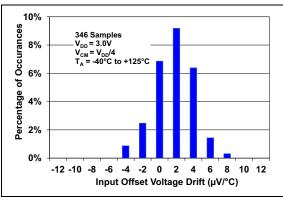
FIGURE 2-2: Input Offset Voltage Drift.
