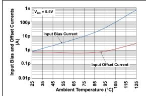
**FIGURE 2-11:** Input Bias, Offset Current vs. Ambient Temperature.
