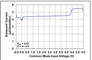
**FIGURE 2-16:** Quiescent Current vs. Common Mode Input Voltage.
