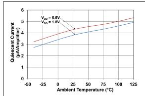
**FIGURE 2-13:** Quiescent Current vs. Ambient Temperature.
