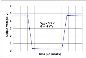
**FIGURE 2-32:** Large Signal Inverting Pulse Response.
