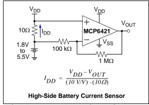
FIGURE 4-10: Battery Current Sensing.
