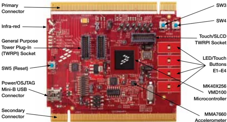
Figure 1: Front Side of TWR-K40X256 Module Not Including TWRPI.
