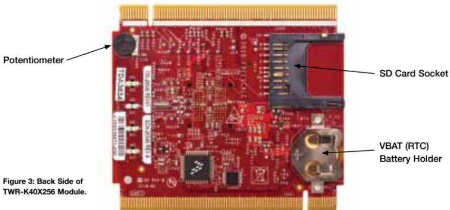
Figure 3: Back Side of TWR-K40X256 Module.
