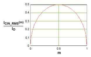
Figure 1. I<sub>CIN</sub> vs. Voltage Conversion Ratio
