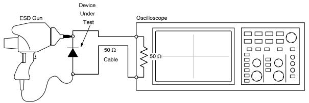
Figure 4. Diagram of ESD Test Setup
