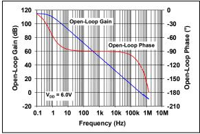
**FIGURE 2-18:** Open-Loop Gain, Phase vs. Frequency.
