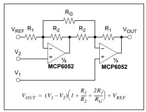
**FIGURE 4-9:** Two Op Amp Instrumentation Amplifier.
