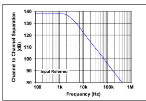
FIGURE 2-21: Channel-to-Channel Separation vs. Frequency (MCP6052/4 only).
