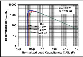
**FIGURE 4-5:** Recommended R<sub>ISO</sub> Values for Capacitive Loads.
