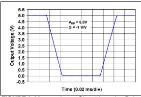
**FIGURE 2-33:** Large Signal Inverting Pulse Response.
