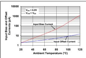
**FIGURE 2-14:** Input Bias, Offset Currents vs. Ambient Temperature.
