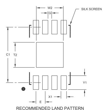
MILLIMETERS Units **Dimension Limits** MIN MOM MAX Contact Pitch Ε 0.50 BSC Optional Center Pad Width W2 1.46 Optional Center Pad Length 1.36 T2 Contact Pad Spacing C1 3.00 Contact Pad Width (X8) X1 0.30 Contact Pad Length (X8) Υ1 0.75 Distance Between Pads G 0.20
