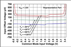
**FIGURE 2-5:** Input Offset Voltage vs. Common Mode Input Voltage with  $V_{DD} = 3.0V$ .
