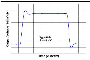
FIGURE 2-30: Small Signal Non-Inverting Pulse Response.
