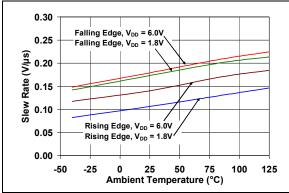
FIGURE 2-29: Slew Rate vs. Ambient Temperature.
