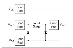
FIGURE 4-1: Simplified Analog Input ESD Structures.
