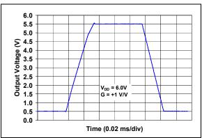
FIGURE 2-32: Large Signal Non-Inverting Pulse Response.
