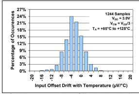
**FIGURE 2-3:** Input Offset Voltage Drift with  $V_{DD} = 3.0V$  and  $T_A \ge +85$ °C.
