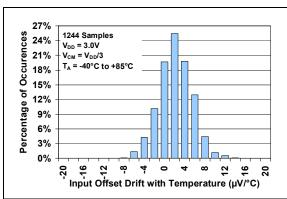
**FIGURE 2-2:** Input Offset Voltage Drift with  $V_{DD} = 3.0V$  and  $T_A \le +85$ °C.
