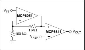
**FIGURE 4-10:** Precision, Non-inverting Comparator.
