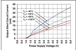
FIGURE 2-25: Ouput Short Circuit Current vs. Power Supply Voltage.
