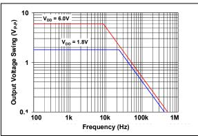
FIGURE 2-26: Output Voltage Swing vs. Frequency.
