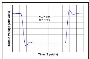
**FIGURE 2-31:** Small Signal Inverting Pulse Response.
