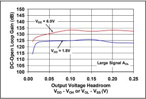
FIGURE 2-20: DC Open-Loop Gain vs. Output Voltage Headroom.
