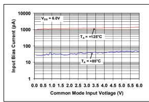
FIGURE 2-15: Input Bias Current vs. Common Mode Input Voltage.
