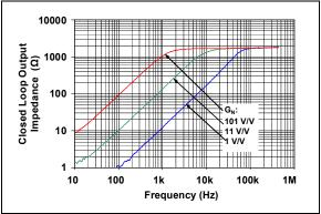
FIGURE 2-35: Closed Loop Output Impedance vs. Frequency.
