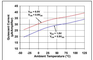
**FIGURE 2-16:** Quiescent Current vs Ambient Temperature with  $V_{CM} = 0.9V_{DD}$ .
