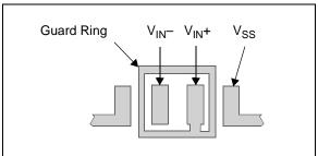
FIGURE 4-7: Example Guard Ring Layout for Inverting Gain.
