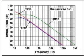
FIGURE 2-11: CMRR, PSRR vs. Frequency.
