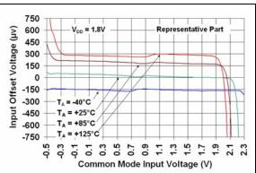
**FIGURE 2-6:** Input Offset Voltage vs. Common Mode Input Voltage with  $V_{DD} = 1.8V$ .
