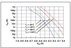
**FIGURE 2-36:** Measured Input Current vs. Input Voltage (below V<sub>SS</sub>).
