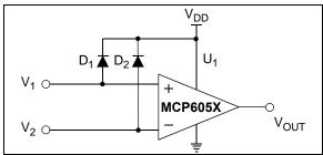
FIGURE 4-2: Protecting the Analog Inputs.
