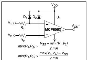
FIGURE 4-3: Protecting the Analog Inputs.
