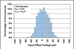
FIGURE 2-1: Input Offset Voltage with  $V_{DD} = 3.0V$ .
