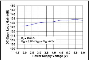
**FIGURE 2-19:** DC Open-Loop Gain vs. Power Supply Voltage.
