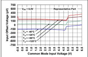
**FIGURE 2-4:** Input Offset Voltage vs. Common Mode Input Voltage with  $V_{DD} = 6.0V$ .
