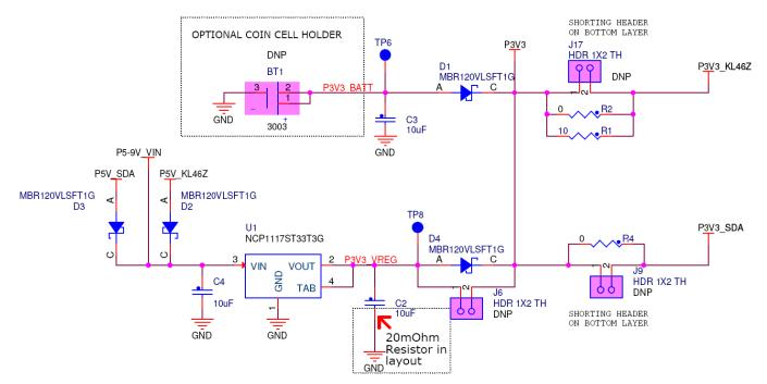
Figure 3- Power Supply Schematic
