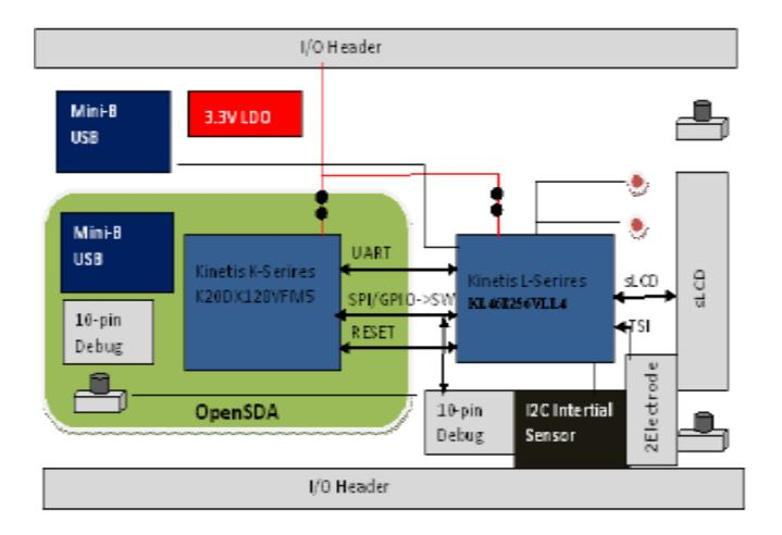
Figure 1. FRDM-KL46Z block diagram
