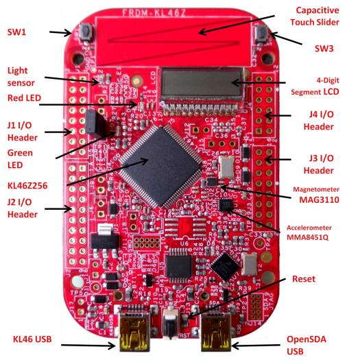
Figure 2. FRDM-KL46Z main components placement.
