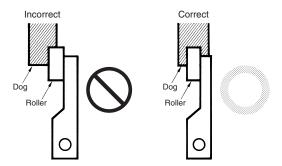
• With a roller actuator, the dog must touch the actuator at a right angle. The actuator or shaft may deform or break if the dog touches the actuator (roller) at an oblique angle.
