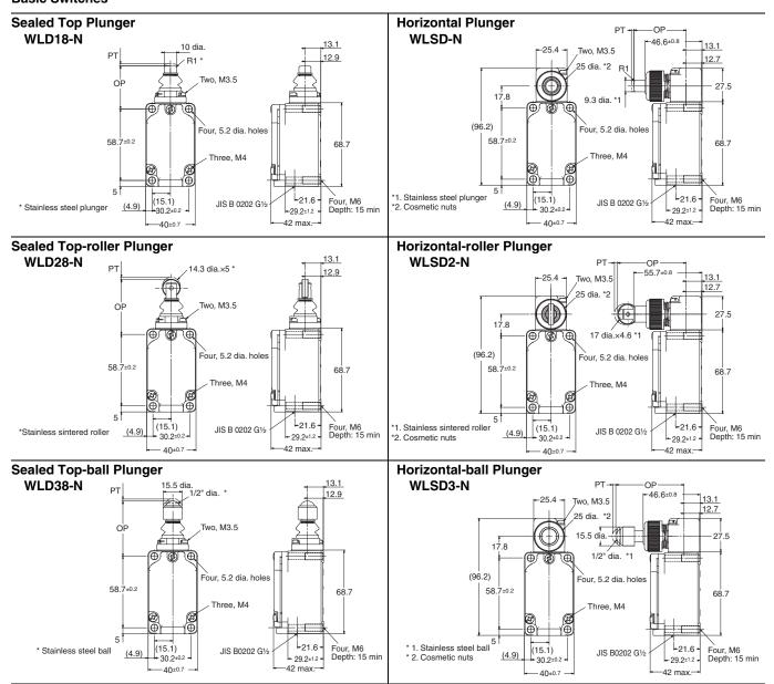
Note: Unless otherwise indicated, a tolerance of  $\pm 0.4$  mm applies to all dimensions.
