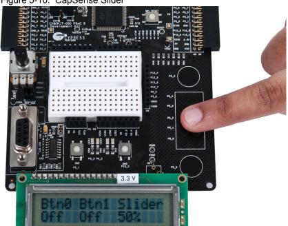
Figure 5-10. CapSense Slider
