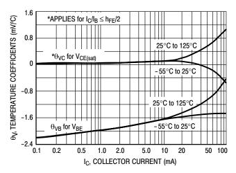
Figure 12. Temperature Coefficients
