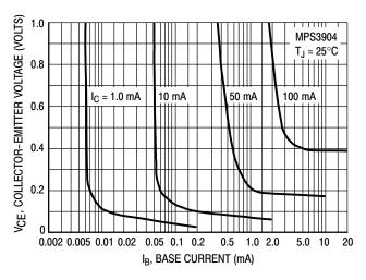
Figure 9. Collector Saturation Region
