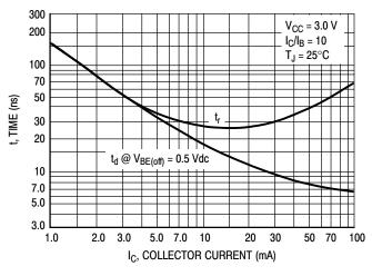
1000 700 500 300 200 t, TIME (ns) 100 70 50  $V_{CC} = 3.0 V$ 30  $I_C/I_B = 10$ 20  $I_{B1} = I_{B2}$  $T_J = 25^{\circ}C$ 10 2.0 3.0 30 70 100 1.0 5.0 7.0 10 50 IC, COLLECTOR CURRENT (mA)
