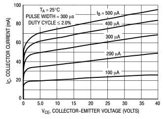
Figure 10. Collector Characteristics
