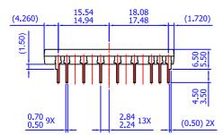
NOTES: UNLESS OTHERWISE SPECIFIED A) THIS PACKAGE DOES NOT COMPLY TO ANY CURRENT PACKAGING STANDARD B) ALL DIMENSIONS ARE IN MILLIMETERS C) DIMENSIONS ARE EXCLUSIVE OF BURRS, MOLD FLASH, AND TIE BAR EXTRUSIONS D) ( ) IS REFERENCE E) [ ] IS ASS'Y QUALITY E) DAMANG EN ENAMEL MODOSCA DEV(2)
