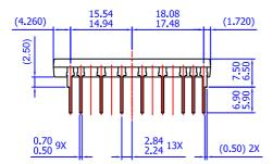
NOTES: UNLESS OTHERWISE SPECIFIED A) THIS PACKAGE DOES NOT COMPLY TO ANY CURRENT PACKAGING STANDARD B) ALL DIMENSIONS ARE IN MILLIMETERS C) DIMENSIONS ARE EXCLUSIVE OF BURRS, MOLD FLASH, AND TIE BAR EXTRUSIONS D) ( ) IS REFERENCE E) [ ] IS ASS'Y QUALITY
