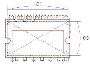
Figure 9. Flatness Measurement Position
