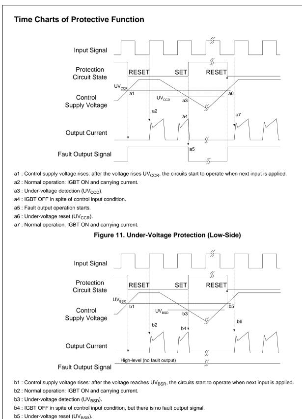
b6 : Normal operation: IGBT ON and carrying current.
