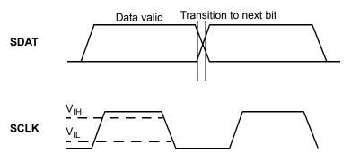
Figure 14. Data Frame Architecture
