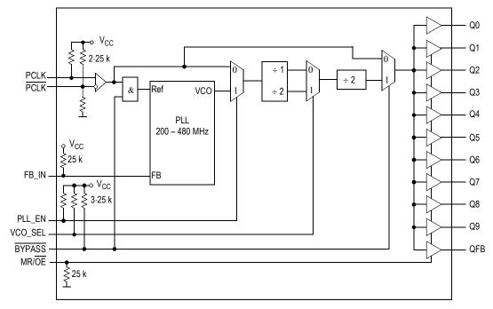
Figure 1. MPC9658 Logic Diagram
