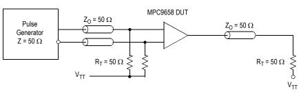
Figure 9. PCLK MPC9658 AC Test Reference
