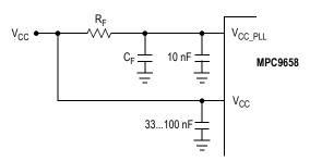
Figure 3. V<sub>CC PLL</sub> Power Supply Filter
