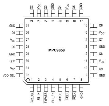
Figure 2. MPC9658 32-Lead Pinout (Top View)
