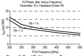
Figure 5. Max. I/O Jitter versus Frequency
