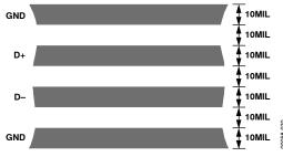
Figure 20. Arrangement of Signal Tracks
