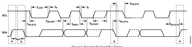
Figure 3. Diagram for Serial Bus Timing
