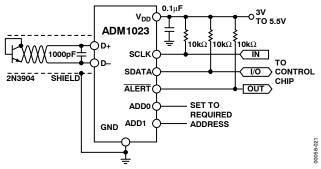
Figure 21. Typical Application Circuit
