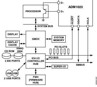
Figure 22. System Using ADM1023 and I/O Controller
