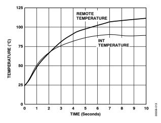
Figure 13. Response to Thermal Shock
