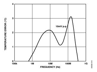
Figure 10. Temperature Error vs. Differential-Mode Noise Frequency
