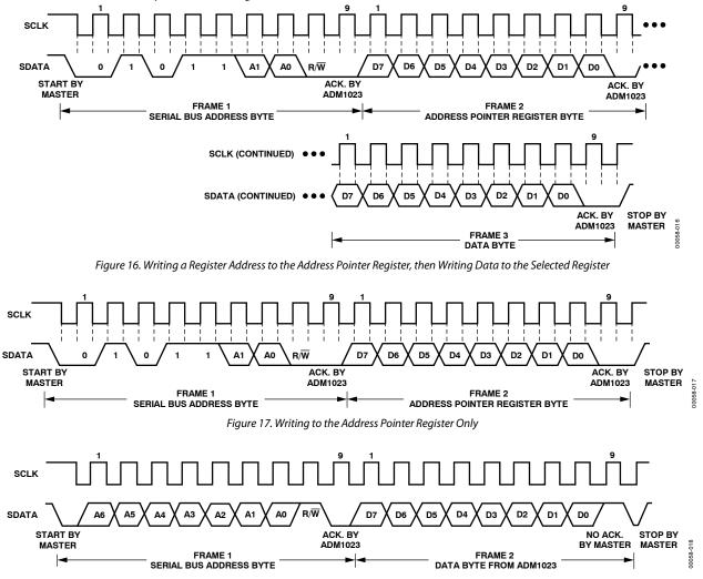
Figure 18. Reading Data from a Previously Selected Register
