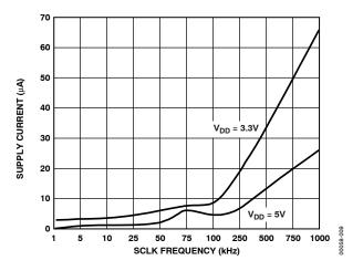
Figure 9. Standby Supply Current vs. SCLK Frequency
