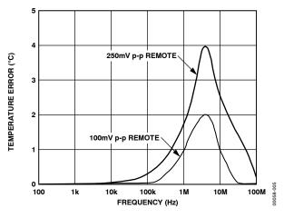
Figure 5. Remote Temperature Error vs. Supply Noise Frequency
