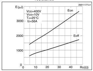
1. Eon including reverse recovery of a SiC diode.
