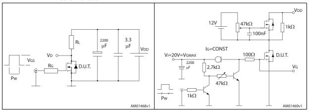
Figure 17. Test circuit for inductive load switching and diode recovery times
