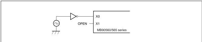
Example of using an external clock
