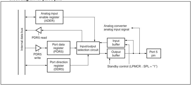
Notes: • When using as an input port, set the corresponding bit in the port 5 direction register (DDR5) to "0" and set the corresponding bit in the analog input enable register (ADER) to "0".
