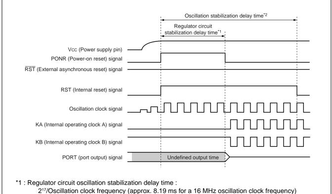
\*2 : Oscillation stabilization delay time :
