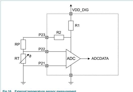
Fig 16. External temperature sensor measurement
