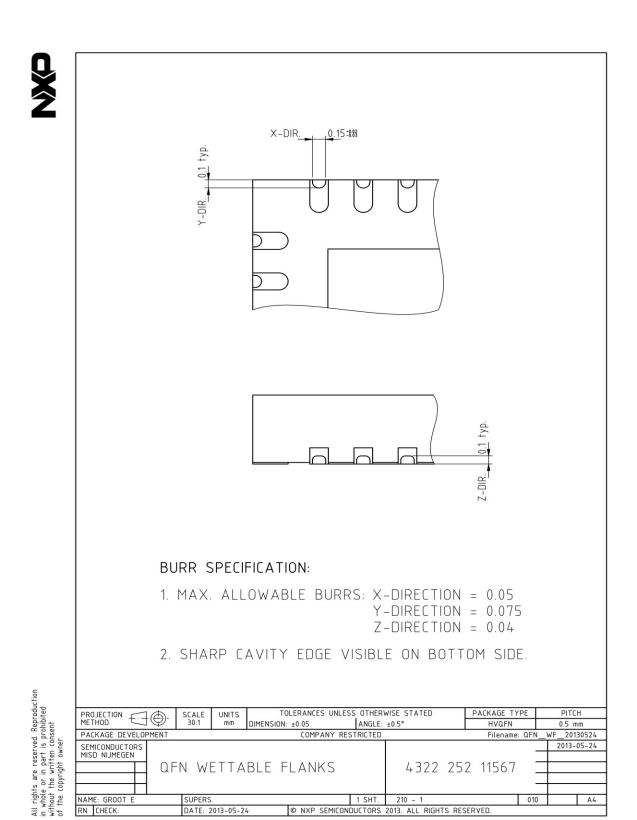
Fig 18. Package detail wettable flanks
