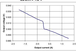
Figure 12. VTT load regulation, 0.75 V, LDOIN = 1.5 V
