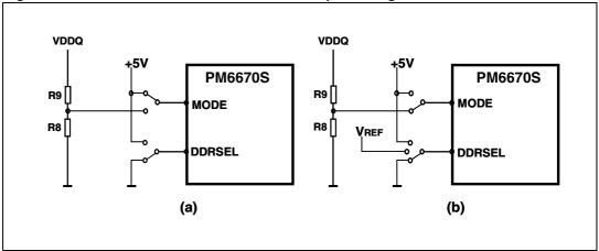
The PM6670S has been designed to satisfy the widest range of applications involving DDR2/3 memories, SSTL15-18 buses termination and I/O supplies for CPU/chipset. The device is provided with multilevel pins which allow the user to choose the appropriate configuration. The MODE pin is used to firstly decide between fixed preset or adjustable (user defined) output voltages.
