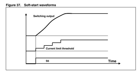
After a fixed 3 ms total time, the soft-start finishes and UVP is released: if the output voltage doesn't reach the under voltage threshold within soft-start duration, the UVP condition is detected and the device performs a soft end and latches off. Depending on the load conditions, the inductor current may or may not reach the nominal value of the current limit during the soft-start (*Figure 38* shows two examples).
