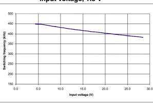
Figure 6. Switching frequency vs input voltage, 1.5 V
