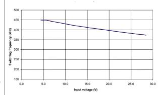
Figure 7. VDDQ line regulation, 1.8 V, 7 A
