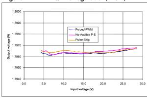
Figure 8. VDDQ line regulation, 1.5 V, 7 A
