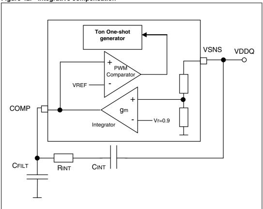
The stability of the system depends firstly on the output capacitor zero frequency. It must be verified that:
