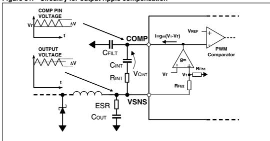
Figure 31. Circuitry for output ripple compensation
