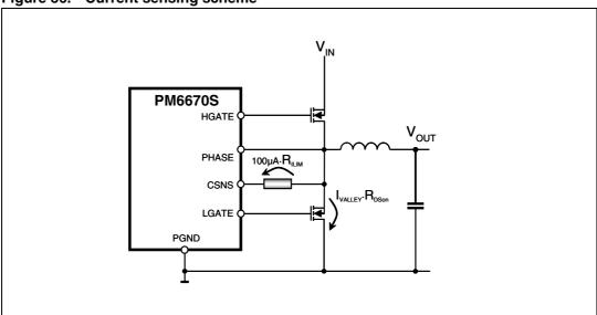
Figure 36. Current sensing scheme
