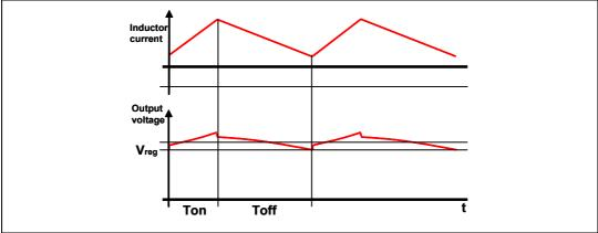
The duty-cycle of the buck converter is, in steady-state conditions, given by
