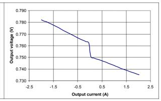
Figure 13. VTTREF load regulation, 0.9 V, VSNS = 1.8 V
