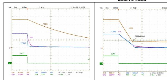
Figure 21. 0 A to 10 A VDDQ load transient, PWM
