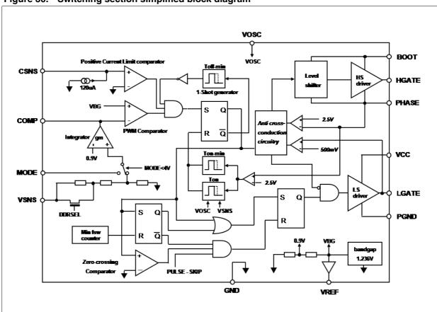
Figure 30. Switching section simplified block diagram
