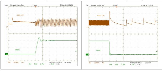
Figure 25. Over-voltage protection, VDDQ = 1.8 V
