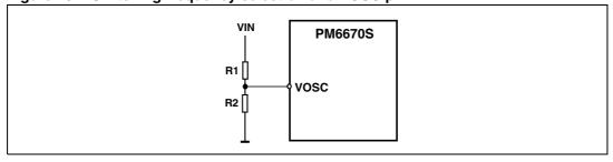
The suggested voltage range for VOSC pin is 0.3 V to 2 V, for better switching frequency programmability.
