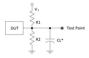
\*CL Includes Test Fixture and Probe Capacitance
