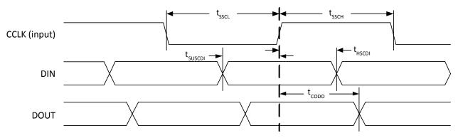
Figure 3.17. sysCONFIG Slave Serial Port Timing
