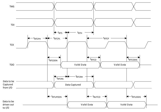
Figure 3.23. JTAG Port Timing Waveforms
