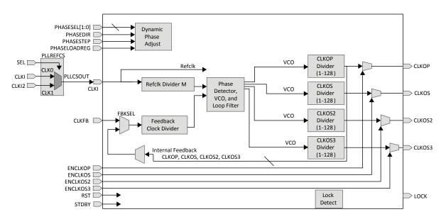
Figure 2.5. General Purpose PLL Diagram
