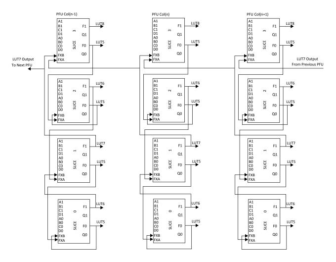
Figure 2.4. Connectivity Supporting LUT5, LUT6, LUT7, and LUT8
