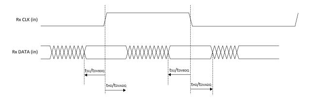
Figure 3.6. Receiver RX.CLK.Centered Waveforms
