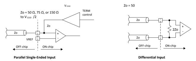
Figure 2.26. On-Chip Termination
