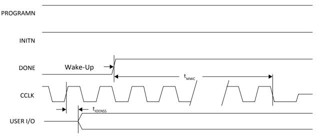
Figure 3.21. Wake-Up Timing
