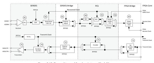
Figure 3.13. Transmitter and Receiver Latency Block Diagram
