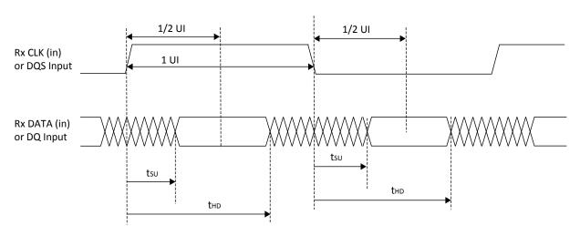
Figure 3.7. Receiver RX.CLK.Aligned and DDR Memory Input Waveforms
