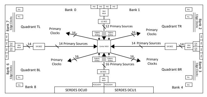
Figure 2.6. LFE5UM/LFE5UM5G-85 Clocking
