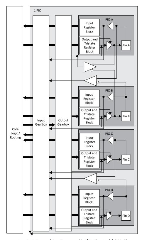
Figure 2.16. Group of Four Programmable I/O Cells on Left/Right Sides
