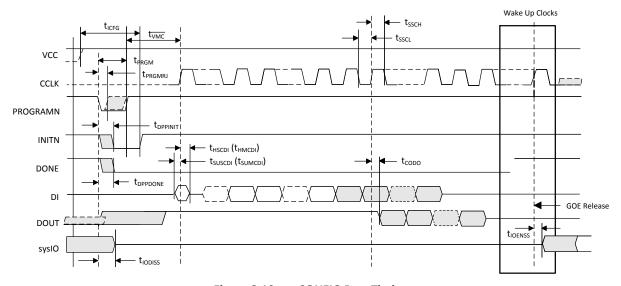
Figure 3.19. sysCONFIG Port Timing
