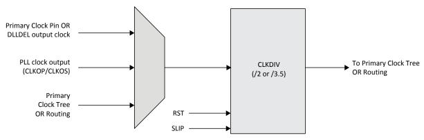
Figure 2.9. ECP5/ECP5-5G Clock Divider Sources
