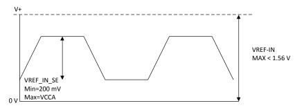
Figure 3.14. SERDES External Reference Clock Waveforms
