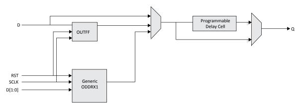
Figure 2.19. Output Register Block on Top Side
