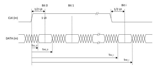
Figure 3.11. Receiver DDRX71\_RX Waveforms
