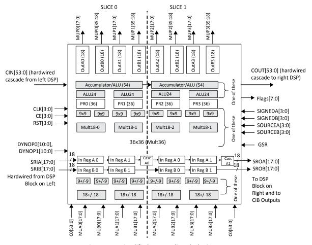
Figure 2.14. Simplified sysDSP Slice Block Diagram
