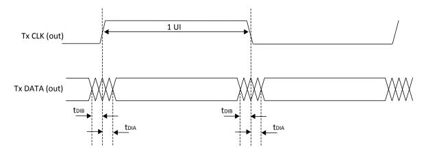
Figure 3.9. Transmit TX.CLK.Aligned Waveforms
