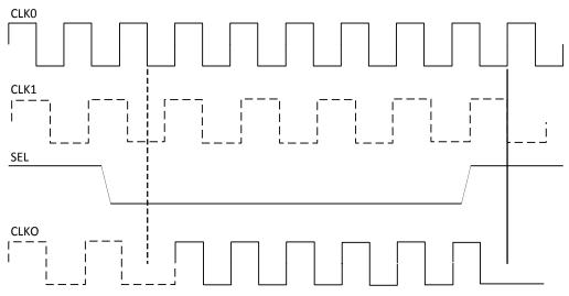
Figure 2.7. DCS Waveforms
