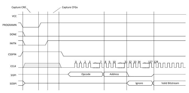
Figure 3.22. Master SPI Configuration Waveforms
