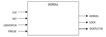
Figure 2.10. DDRDLL Functional Diagram
