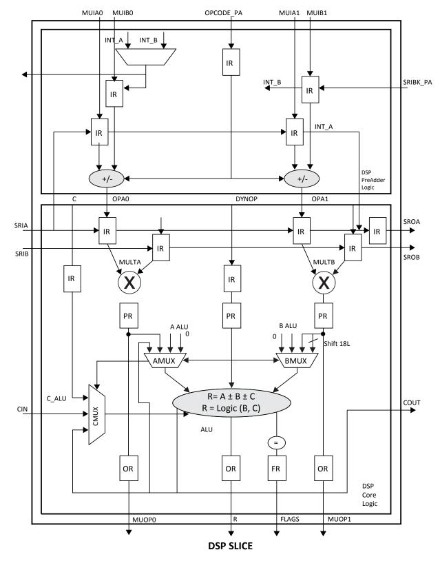
Figure 2.15. Detailed sysDSP Slice Diagram
