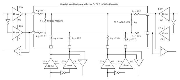
Figure 3.4. MLVDS25 (Multipoint Low Voltage Differential Signaling)
