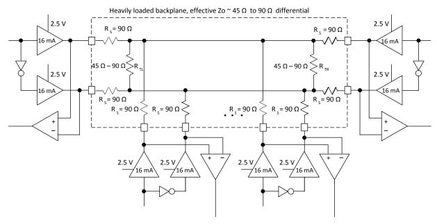
Figure 3.2. BLVDS25 Multi-point Output Example
