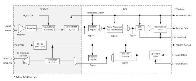
Figure 2.28. Simplified Channel Block Diagram for SERDES/PCS Block
