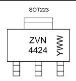
ZVN 4424 = Product Type Marking Code YWW = Date Code Marking Y or  $\overline{Y}$  = Last Digit of Year (ex: 5= 2015) WW or  $\overline{W}W$  = Week Code (01~53)
