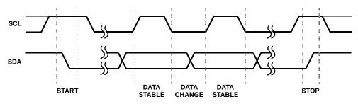
FIGURE 12. VALID DATA CHANGES, START, AND STOP CONDITIONS
