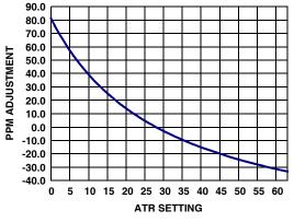
FIGURE 19. ATR SETTING vs OSCILLATOR FREQUENCY ADJUSTMENT
