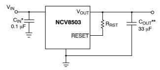
\*C<sub>IN</sub> required if regulator is located far from the power supply filter
