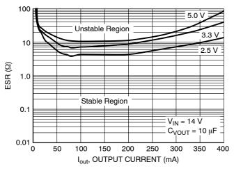
Figure 9. Output Stability with Output Voltage Change
