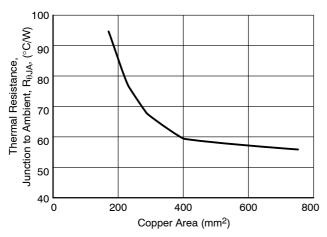
Figure 22. 16 Lead SOW (Exposed Pad),  $\theta$ JA as a Function of the Pad Copper Area (2 oz. Cu Thickness), Board Material = 0.0625" G-10/R-4
