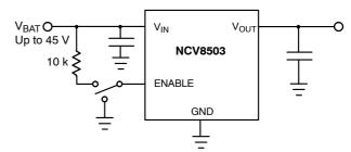
Figure 17. ENABLE Function
