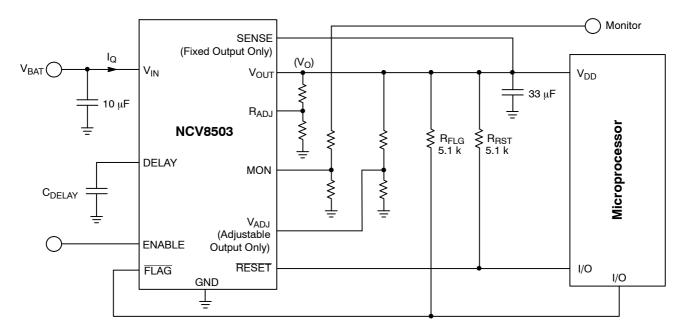
Figure 1. Application Diagram
