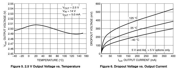
Figure 5. 2.5 V Output Voltage vs. Temperature
