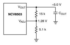
Figure 19. Adjustable Output Voltage
