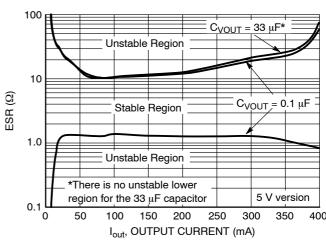
Figure 10. Output Stability with Output Capacitor Change
