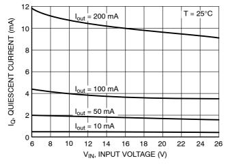
Figure 13. Quiescent Current vs. Input Voltage
