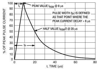
Figure 1. 8 x 20 µs Pulse Waveform
