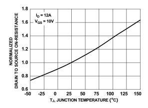
Figure 3. Normalized On-Resistance vs Junction Temperature
