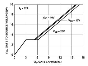
Figure 7. Gate Charge Characteristics
