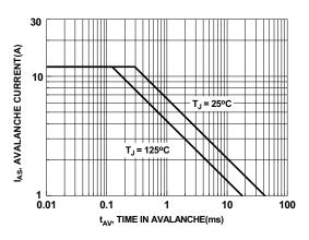
Figure 9. Unclamped Inductive Switching Capability
