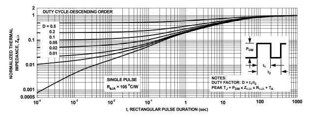
Figure 13. Junction-to-Ambient Transient Thermal Response Curve
