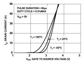
Figure 5. Transfer Characteristics
