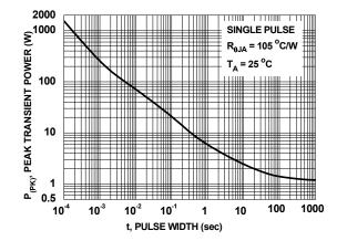
Figure 12. Single Pulse Maximum Power Dissipation
