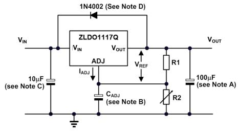
Figure 2. Adjustable Regulator with IADJ Errors
