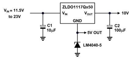
Figure 3. ZLDO1117Q with Extended Output Voltage
