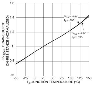
Figure 6 On-Resistance Variation with Temperature
