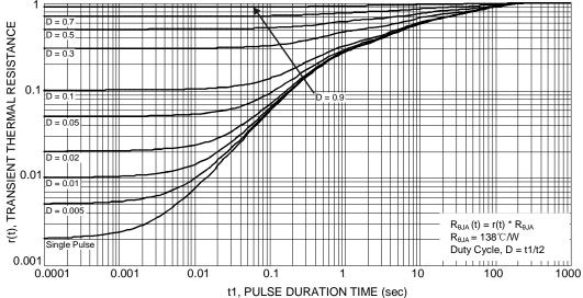
Figure 13 Transient Thermal Resistance
